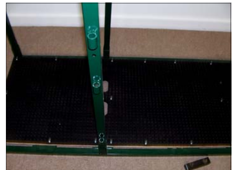
3) Insert the 2 vertical bars with the large bushings and one hole midway up in the middle pipe sockets.
