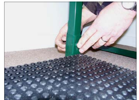
6) Hand tighten the ½" nuts on the outside of the chute.
