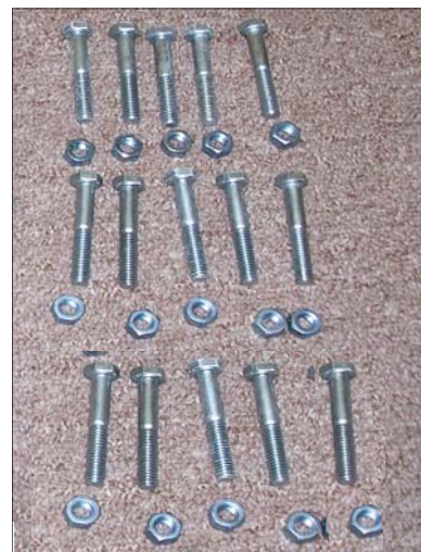
___ 16 bolts & nuts (1/2") for vertical bars & headstall bar
