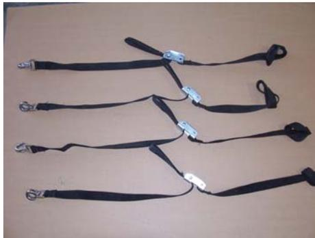
\_\_\_ 4 leg restraint straps (with snap rings)
